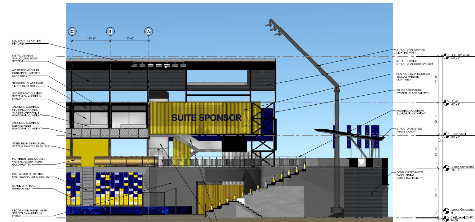
1 INTERIOR EAST ELEV - MATERIAL REFERENCE #1 1/8" = 1'-0"
