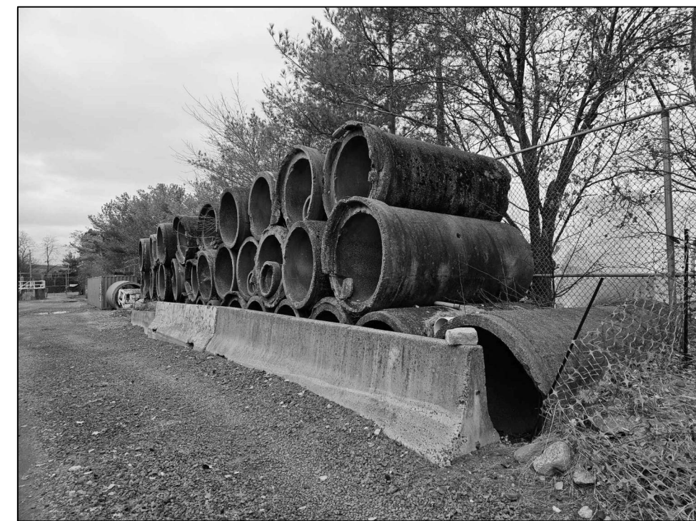
IMAGE 2: STORED REINFORCED CONCRETE PIPES NEXT TO WESTERN FENCE LINE
