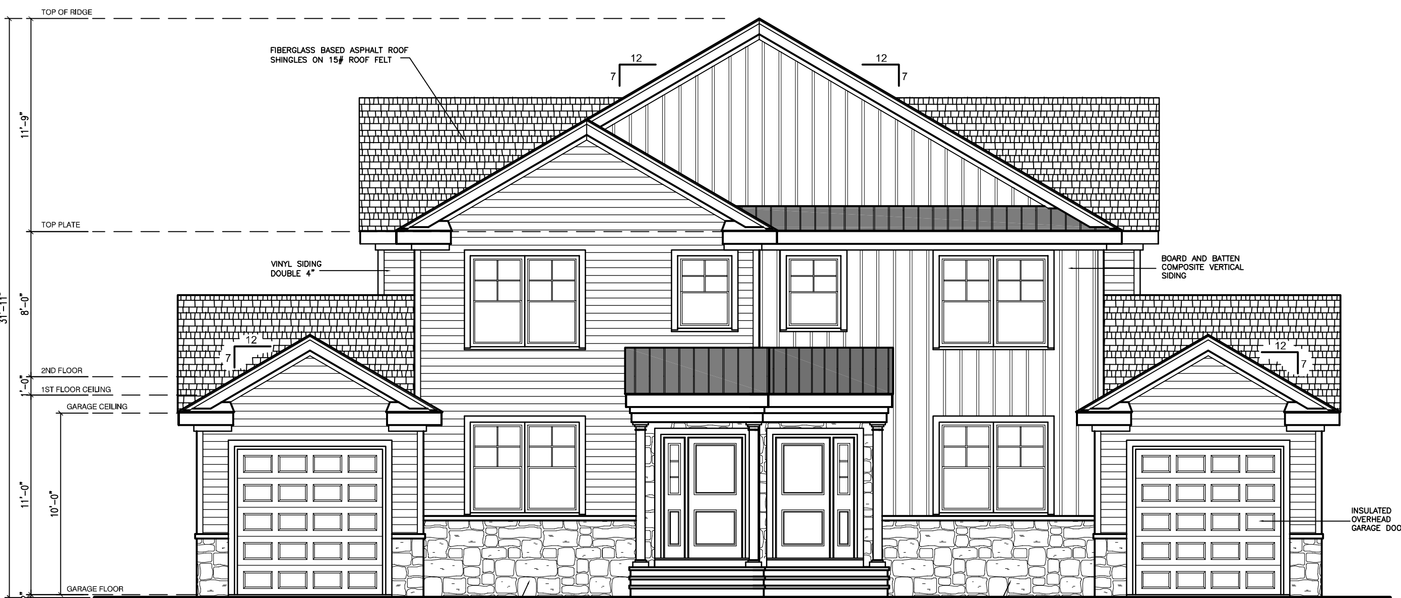
FRONT ELEVATION SCALE 3/8" = 1'-0"
