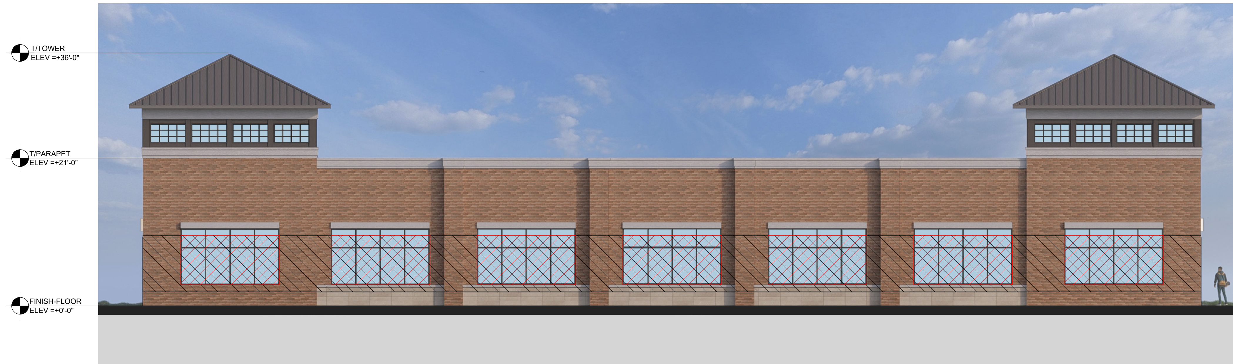
SOUTH ELEVATION (FRONT FACADE) TOTAL FACADE (BETWEEN 2' & 10') 1,200 SF TOTAL GLAZING 686 SF TRANSPARENCY PERCENTAGE 57% TRANSPARENCY REQUIRED 12%
