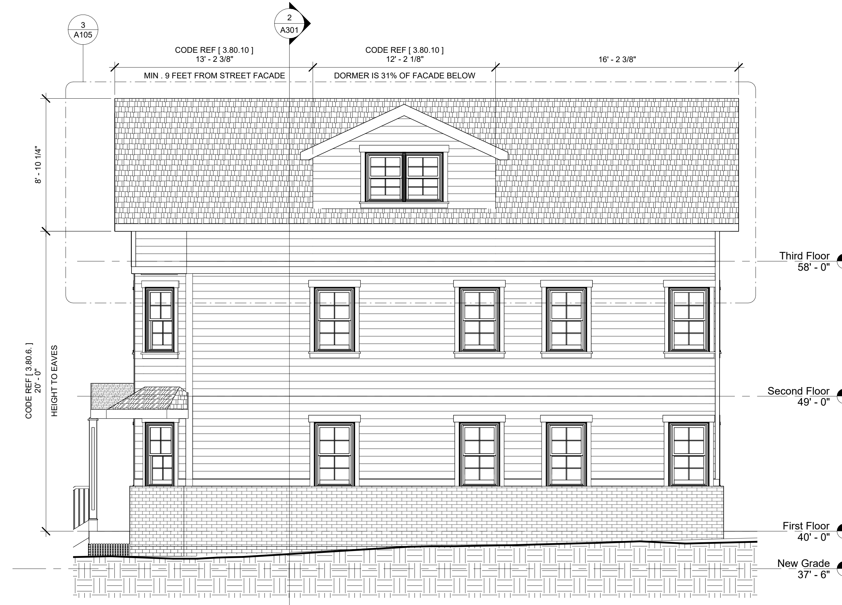
254 Scofield Ave - Double House A - South Elevation 1/4" = 1'-0"
