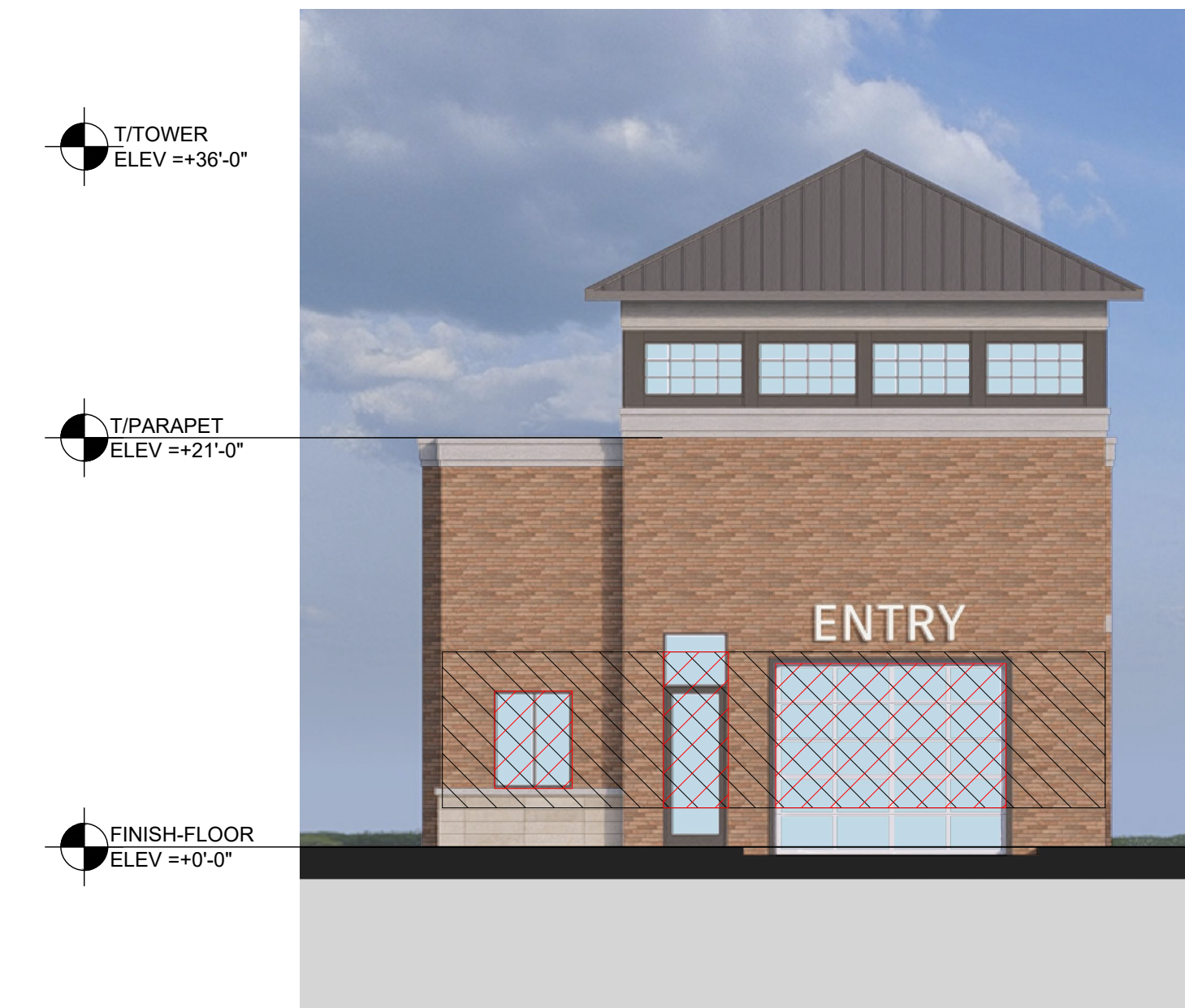
WEST ELEVATION (SIDE FACADE) TOTAL FACADE (BETWEEN 2' & 10') 271 SF TOTAL GLAZING 134 SF TRANSPARENCY PERCENTAGE 49% TRANSPARENCY REQUIRED N/A
