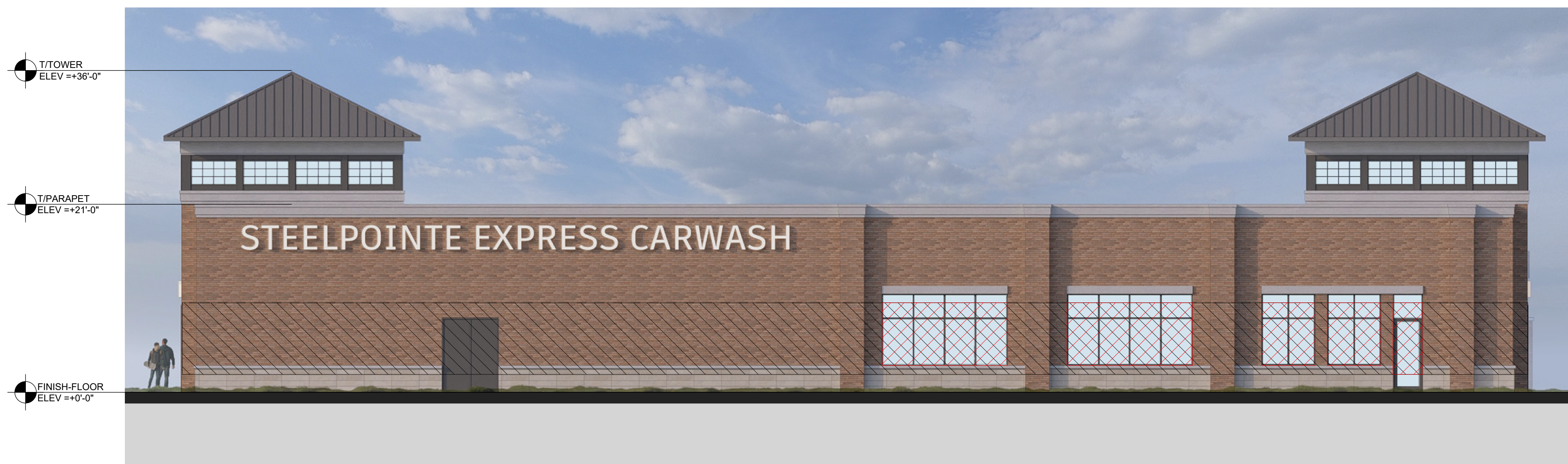
NORTH ELEVATION (REAR FACADE) (FACING I-95 EXIT RAMP) TOTAL FACADE (BETWEEN 2' & 10') 1200 SF TOTAL GLAZING 307 SF TRANSPARENCY PERCENTAGE 25% TRANSPARENCY REQUIRED 12%
