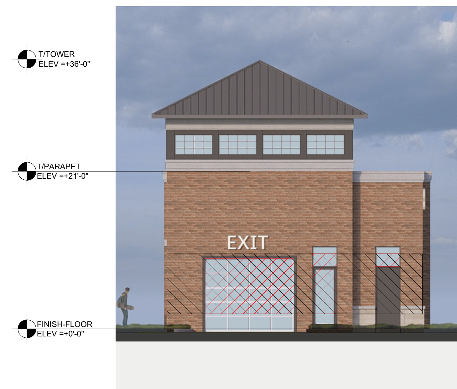
EAST ELEVATION (SIDE FACADE) TOTAL FACADE (BETWEEN 2' & 10') 271 SF TOTAL GLAZING 119 SF TRANSPARENCY PERCENTAGE 44% TRANSPARENCY REQUIRED N/A
