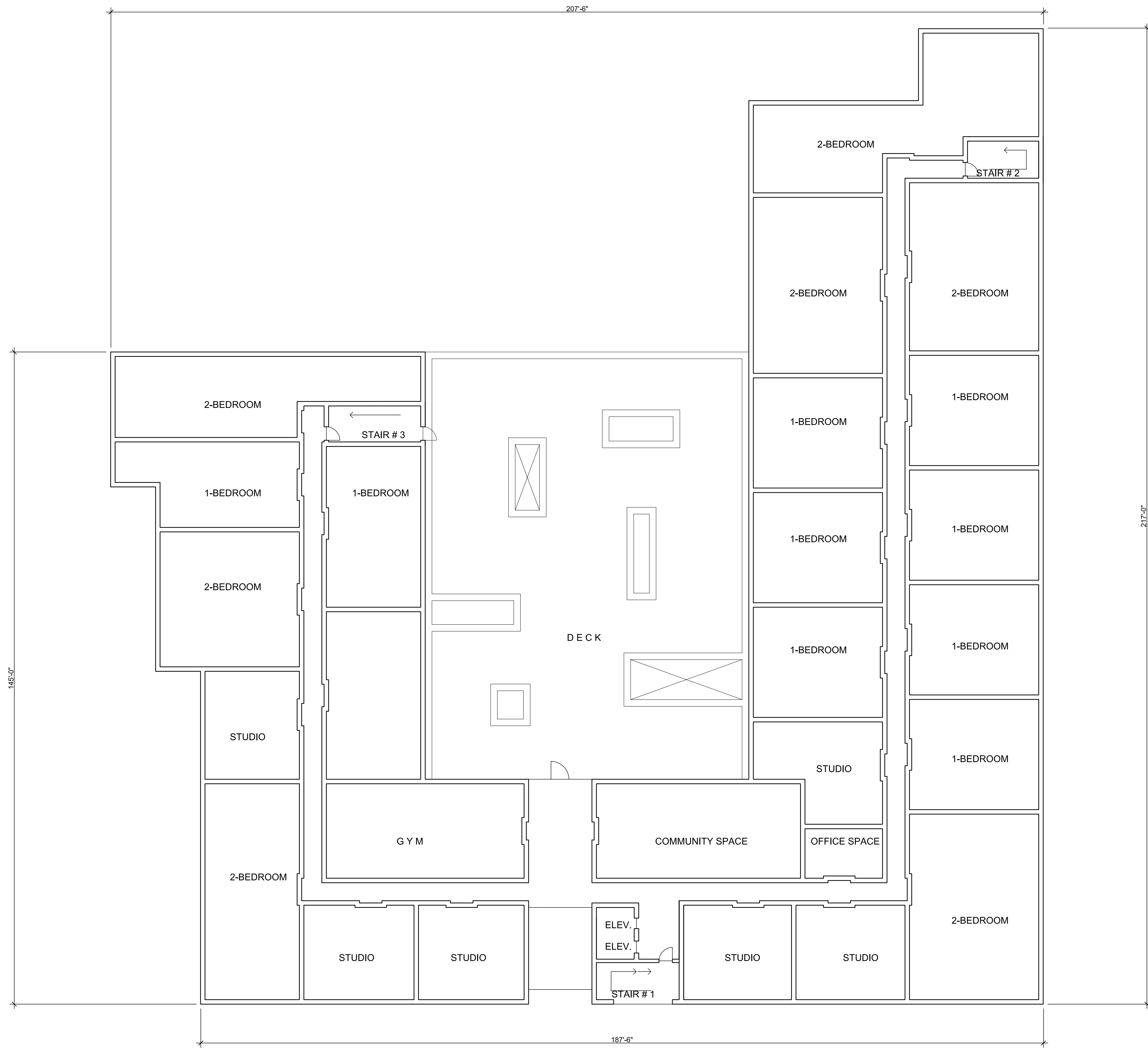
1 SECOND FLOOR PLAN SCALE: 3/32"=1'-0"
