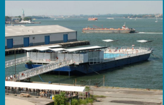
The Floating Pool Lady is a barge converted to a floating pool by the NYC Department of Parks and Recreation. Image Source: Jonathan Kirschenfeld
