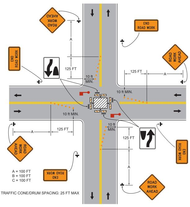
WORK AREA CAN BE ADJUSTED TO ACCOMMODATE WORK LOCATION
